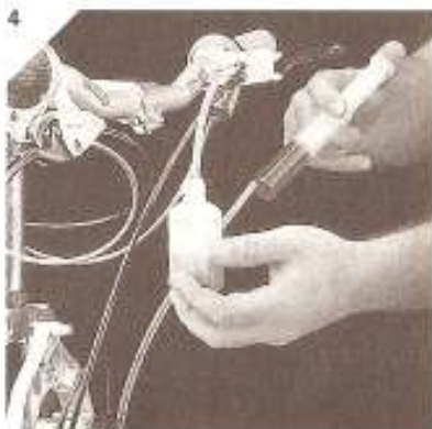
4 Fill the syringe only with hydraulic oil. Only use mineral oil! Never use car brake fluid. Even sewing machine oil is fine.
